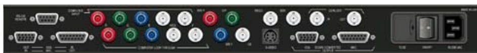
Back Panel Drawing of Scan Do Ultra/D (There is no SDI BNC connector on Scan Do Ultra)
